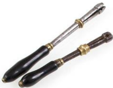
Early 19th century hand vices. Hardy's were using bench mounted versions of these vices in when they closed their fly shop in 1969. Salmon flies were still tied without a vice at that time.
