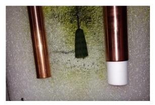
You start with a chunk of high density foam out of which must emerge a foam cylinder of a desired diameter and length. Anyone who has tried to use a punch to do this will tell you how unfortunate the result can be. Dustan uses a piece of copper plumbers pipe of the desired diameter sharpened on one edge. This is the cutting edge which is twisted into the foam thus cutting the desired cylinder. You can do it by hand or attach the tube to a drill. Both work equally well.
